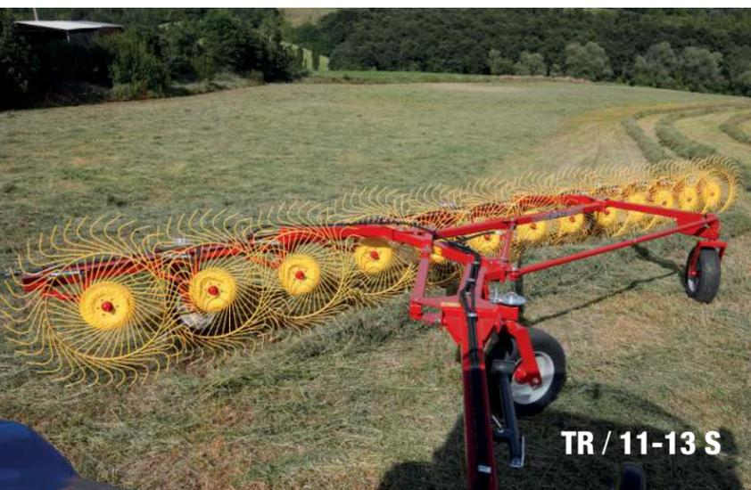
The new range of TR/6-13S in-line trailed wheel rakes stands out from the traditional earlier range for its smaller transport dimensions and for being extremely easy to use and to adjust while working. The machine can be moved from the transport to the working position and back to the transport position from the tractor, using the hydraulic system. The machine's sturdy design provides excellent performance both in terms of quantity and quality.
