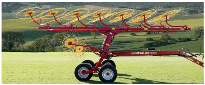
The actuator selector (angulation - extension) makes it possible to quickly adjust the working width and windrow width from the tractor distributor.
